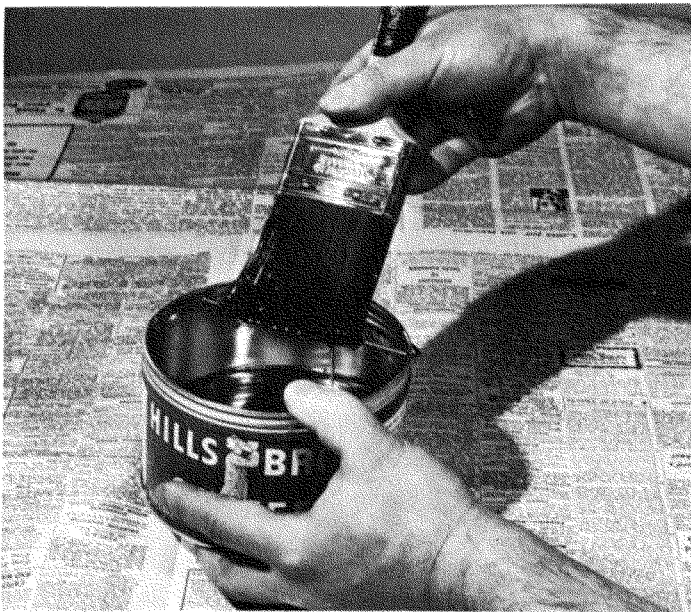
Fig. 707. Technique used when applying lacquer with a brush: a) remove excess lacquer from the brush to aid in producing an even spread; b) apply lacquer in direction of grain. Note the proper way to hold the brush.
