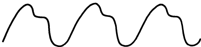
Fig. 302. When a wave contains a harmonic it becomes complex. Although this waveform is not smooth it repeats at regular intervals.
